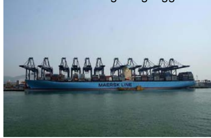
In 2006 the largest containership ever built, Emma Maersk, was launched with a reported capacity of 12,508 TEU capacity she requires a depth of 16 metres 156,907 DWT (carrying capacity)
